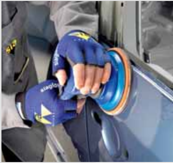
Producing a mat finish on painted surfaces
