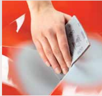
Final sanding of filler at hard to get at areas
